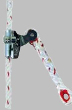
This sliding fall arrester has an automatic locking function and a guide mechanism. This fall arrester moves along the anchor line, accompanying the user while moving up and down the line with no need for any manual intervention and it automatically locks onto the anchor line in case of a fall, with the corresponding dissipation of energy. The dissipation takes place due to the joint action of the sliding fall arrest device and the anchor line.
